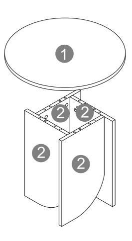
STEP 1: Fix dowel (B) and cam pin (A) to panel (1)(2).
